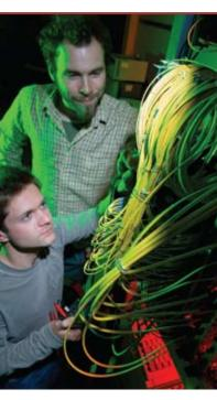
A researcher and a PhD student work together to cable and test some of the readout electronics of CMS.
